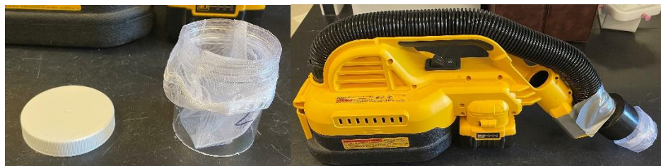
Figure 2. Whitefly sampling device. Mesh bags are fitted over 2.5inch diameter jars with the bottoms removed, which are then affixed to the tube of a battery powered industrial hand vacuum. After sampling from foliage for a set period of time, the cap is placed over the jar lid to contain the insects for later counting.
